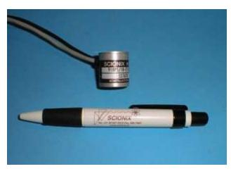
The signals need to be processed by a follow-up amplifier. The lowest energy that can be detected is 40 keV.
