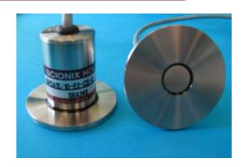
Csl(Tl) crystals provide the highest signal to noise ratio of all scintillators operated in pulse counting mode due to the fact that the emission is located in the yellow part of the spectrum where the quantum efficiency of photodiodes is highest.
