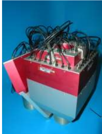
Examples of BGO shields in nuclear spectroscopy
