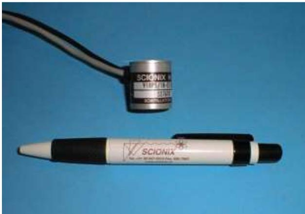
The signals need to be processed by a follow-up amplifier. The lowest energy that can be detected is 40 keV.
