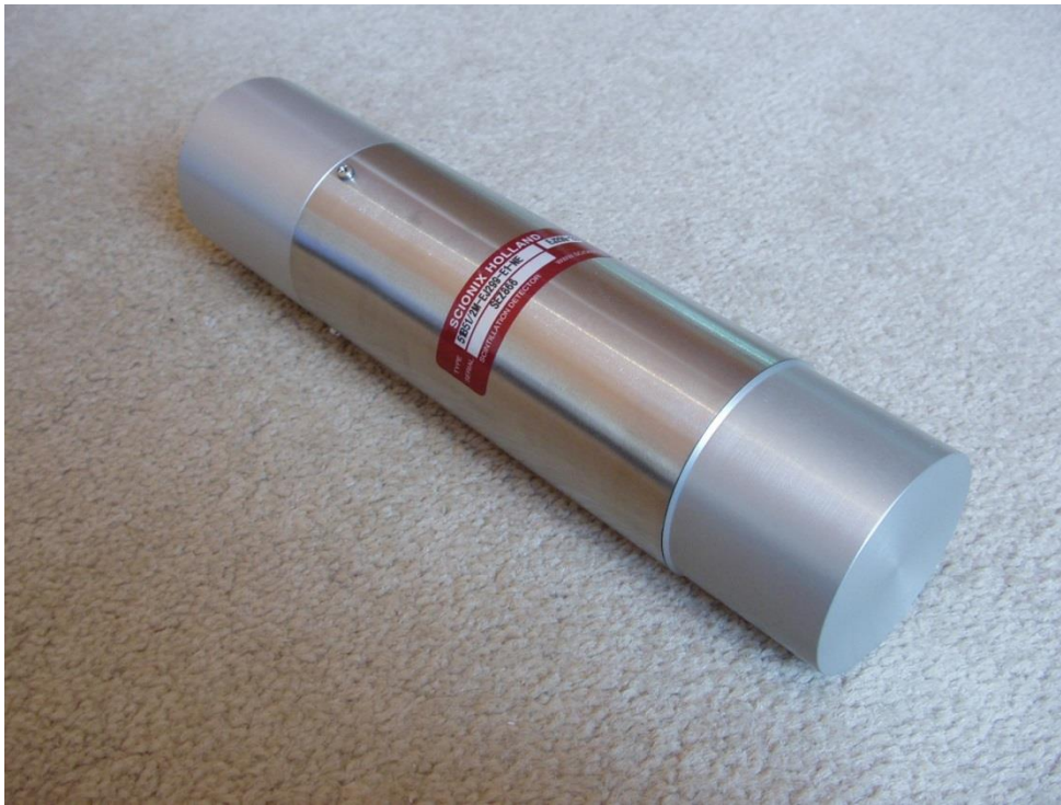
EJ299-33 scintillation detector with fast 2 ns PMT and transistorised voltage divider
