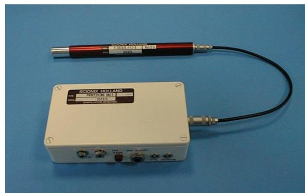
The signal and power supply junction box provides the high voltage to the probe and processes the analog signal from the PMT.
